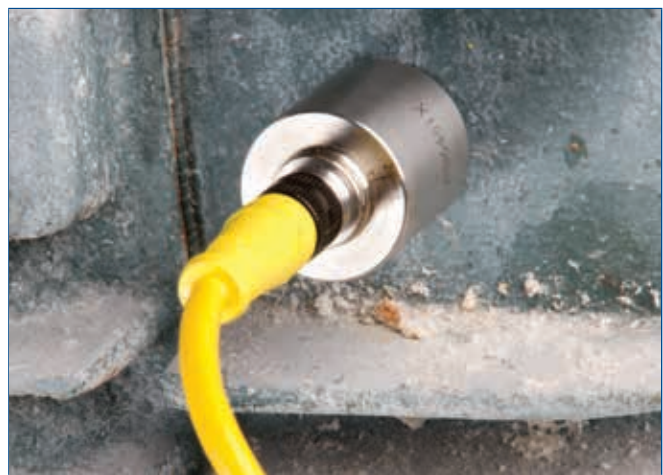
The triaxial accelerometer collects data at the measurement location from a vertical, horizontal, and axial directions simultaneously.
