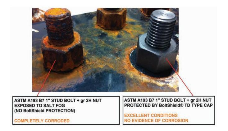
ASTM B-117 is an accelerated salt fog test recognized worldwide.
